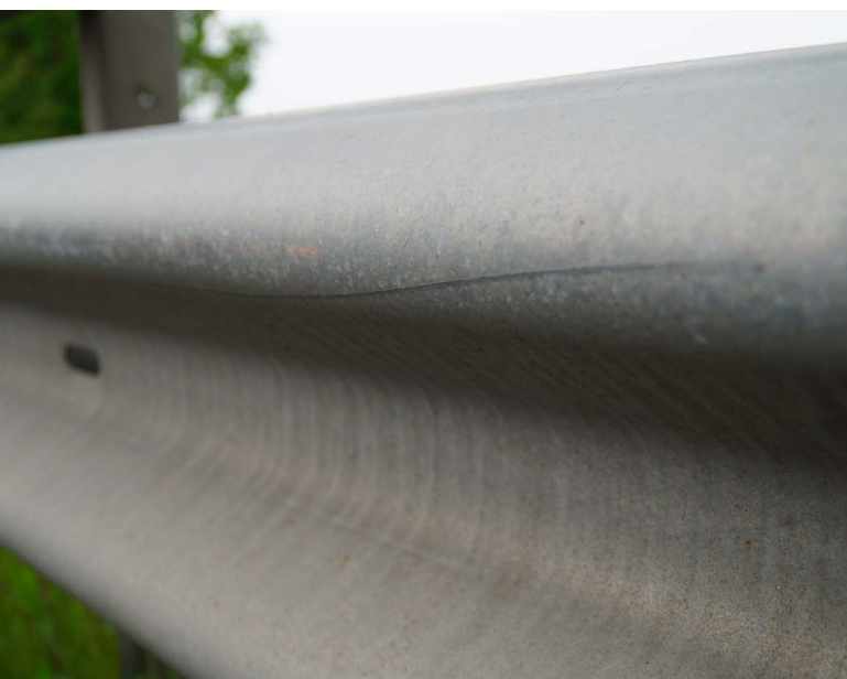
Fig. 3: Thin-film “microZINQ®”-galvanized crash barrier with a collision mark.
